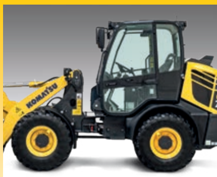
Low total height (2,48 m) for easy transport
