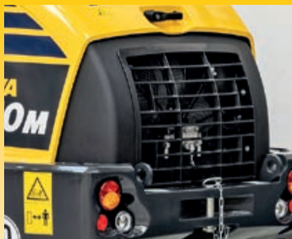
Wide core radiator with (optional) reversible fan
