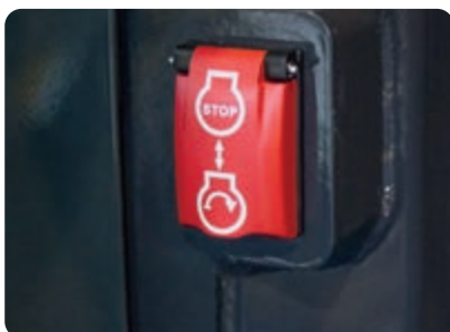
Secondary engine shutdown switch
